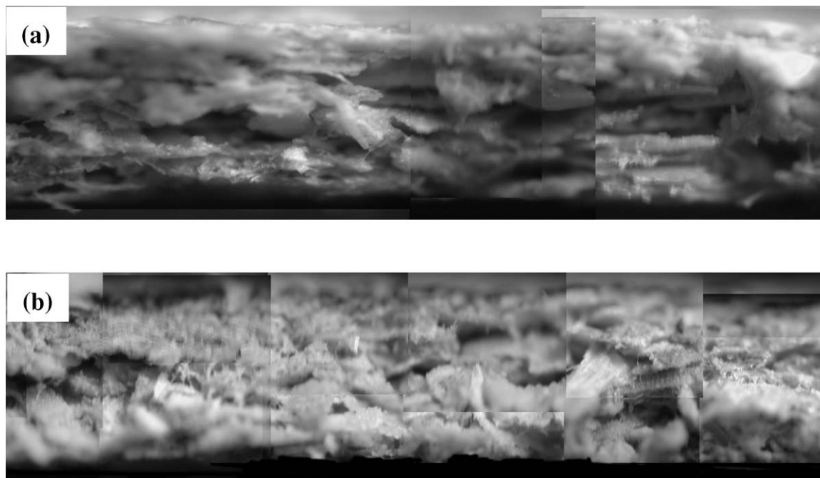
Figure 2 The optical micrographs of the cross-sectional structures of the RPC sheets (40 \times ) fabricated: (a) with the conventional rolling technique and (b) the novel 3D rolling methodology.
